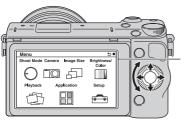
When options are displayed on the screen, you can browse through them by turning or pressing the top/bottom/left/right parts of the control wheel. Press the center to make your choice.
