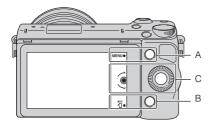
In this case, soft key A works as the MENU (Menu) button, and soft key B as the 1 (Send to Smartphone) button.
